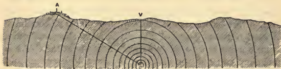
FIG. 39.—Diagram-section to illustrate the propagation of an earthquake-wave and the mode of calculating the depth of its origin.
